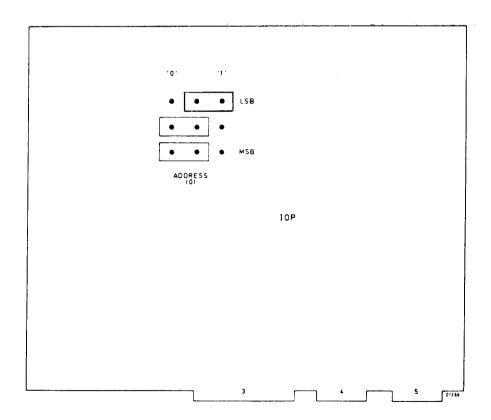
Figure 12.1 IOP/MX ADDRESS STRAPS
