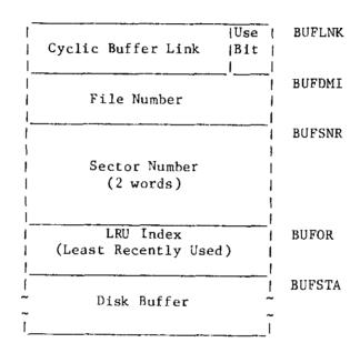
The words BUFDMI and BUFSNR define one unique sector. The LRU index is kept in the buffer header to let buffers remain in memory as long as possible in order to minimize physical I/O. The word CURBUF contains a pointer to the current buffer.
