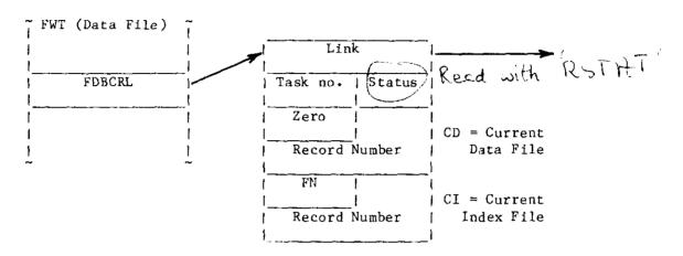
One CRN buffer (6 words) is allocated for each user task per file structure (data file with/without index file). Other data management requests from the same task to the same structure will use the same CRN buffer. The buffer is released after closing the file. When more than one task is using the same file structure, the CRN buffers are linked via the first word in the buffer.
