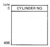
A cylinder number is written in the first word of every sector when the disk is initially formatted by the utility PM6800. It contains the number of the cylinder in which the sector is located. It is used by the Monitor to check if a seek operation has been successful or not.
