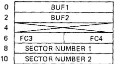
BUF1: Address of the disk sector buffer BUF2: Address of the print buffer FC3: File code of the print device
