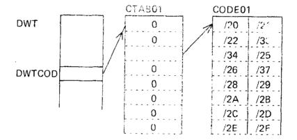
DWTCOD of the device work table holds an address of an 8word table CTAB01, indicating the columns to be converted. (DWTCOD) = 0 means no conversion for this keyboard.
